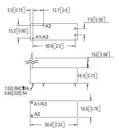
(1) PC pin versions carry 5 or 10 amps, see part number system. Flying lead and panel versions carry 10 amps.
